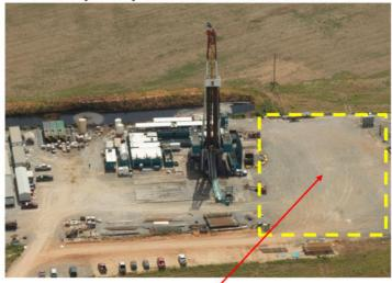
Space available for frac operations while simultaneously drilling on the same pad
