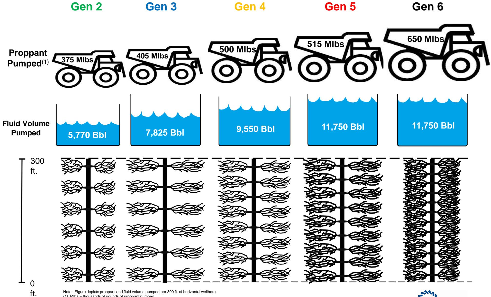
Note: Figure depicts proppant and fluid volume pumped per 300 ft. of horizontal wellbore.
